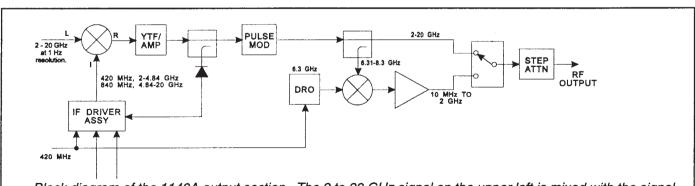
Block diagram of the 1140A output section. The 2 to 20 GHz signal on the upper left is mixed with the signal from the IF Driver to produce the output frequency. For complex modulation, this IF driver signal uses a front panel input.
